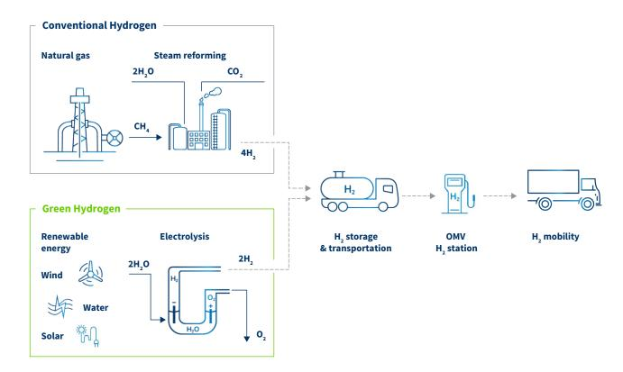
In conventional hydrocarbon-based hydrogen production, we are looking into ways to prevent  $CO_2$  produced in the steam-reforming process from being expelled as emissions. Instead, we aim to capture it and use it as a feed-stock for producing methanol. This is then further turned into renewable-based chemicals and fuels.
