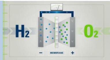
The end product from the chemical reaction is power for the drive train and H2O, i.e. pure water. This is the only emission produced by this mini power station.
